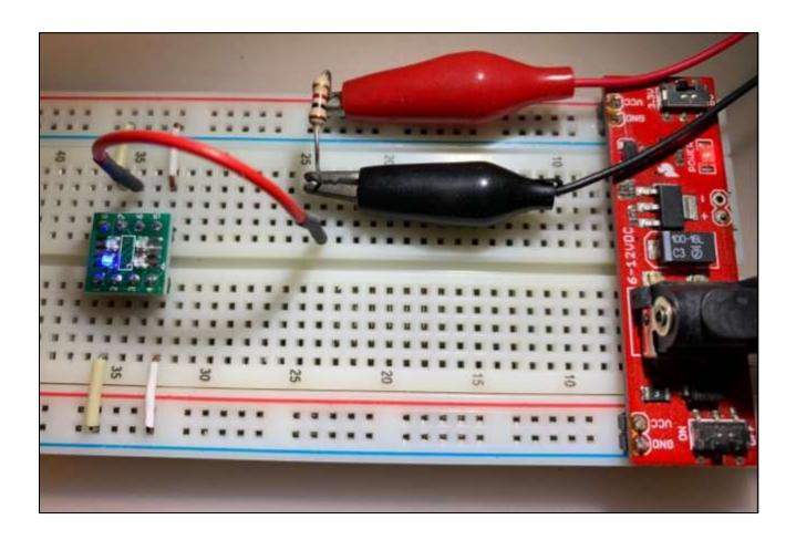
Using this setup, it was easy to select the LED, supply voltage, resistance. I chose a range of resistance values from 200 to 3300 ohms, thus varying the current through the LED.
