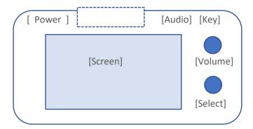
Another design consideration was the SD card slot. Although I attempted to remove as much dependency on pre-built modules, the Chinese-manufactured 3.2" display (with built-in SD card holder) is tough to beat. Soldering up and mounting your own TFT display is challenging. So, I stuck with the MSP3218-style board. This board places the SD card on top - see dotted rectangle above. The SD card
