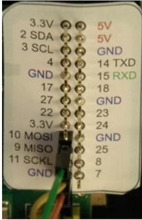
connector” to find mating connectors, which cost about \$0.50 each. With a little care, even oversized, 40-pin computer ribbon cables can be attached. This project only needs four wires, so I used individual female-to-male breadboard jumper wires.
