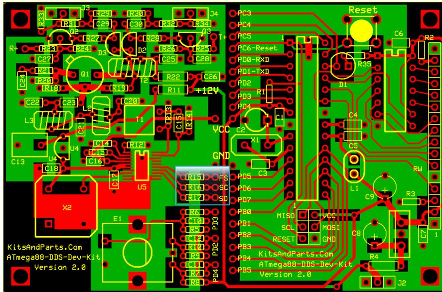
The DDS board is really two boards in one: the left half of the board contains the DDS and analog output circuitry; the right half is the ATmega88 microcontroller and its supporting components. The center of the board is literally two rows of holes allowing connections between the two. Nearly all of the ATmega88 I/O lines are brought out for our
