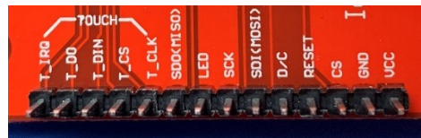
14 pins, with the first 5 labelled as touch
